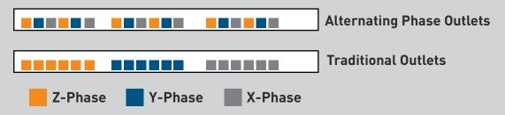
Power wiring becomes much more simplified with this type of PDU since power cords do not need to be stretched across the length of the vertical PDU to reach separate branches. Plugging into a different phase only means moving the cord several inches to the next available receptacle. Shorter power cords from the server to the PDU can now be used thus cleaning up the back of the rack cabling.
